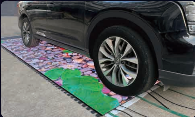
Car load-bearing test 1m 2 load capacity 1000kg
